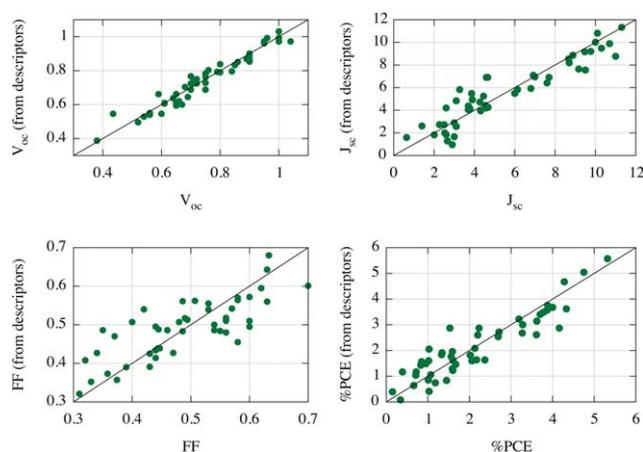
**Fig. 3** Results for the multiple linear regression of the four models and the values of the training set. The predicted value from fitted descriptors is compared to the experimental value originally used for fitting. Units are  $\text{mA cm}^{-2}$  for  $J_{sc}$ , and V for  $V_{oc}$ .
