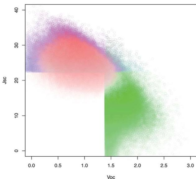
**Fig. 5** Top 10% molecules with highest predicted values of  $V_{oc}$  (green),  $J_{sc}$  (blue), and  $V_{oc}J_{sc}$  (red). The intensity of the point corresponding to a given molecule is coded according to the value of the product  $V_{oc}J_{sc}$ . The best molecules, according to the present study, are located in the upper left region of the figure. Units are mA cm<sup>-2</sup> for  $J_{sc}$ , and V for  $V_{oc}$ .
